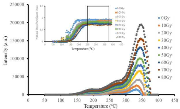
Figure 3. Thermoluminescence (TL) intensity responses as functions of temperature for SH1 subsamples exposed to different doses (Gy).
